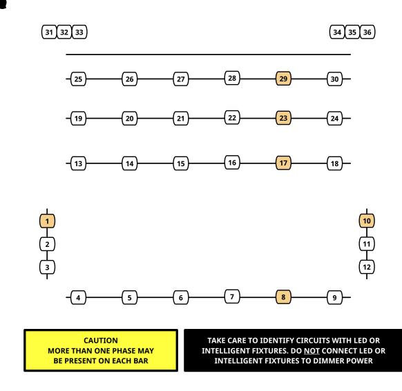
The outlets highlighted in **Amber** are typically patched to provide hard power to intelligent and LED fixtures, and are not generally available for patching to dimmers.
